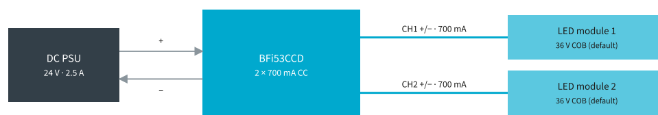
Figure 2: Dual constant-current wiring
